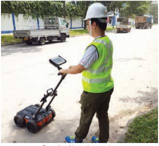
Ground probing radar scanning
